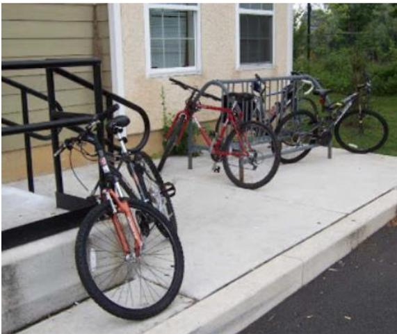
Figure 1. Older style of bicycle rack, colloquially known among cyclists as a “wheel bender.” Note how bikes have been locked to the ends of the rack to avoid the wheel-bending effect, and one cyclist has avoided using the rack altogether. Source: First State Bikes (<http://www.1stbikes.org/2013/05/youtube-video-ban-wheelbender-bike-rack.html>).
