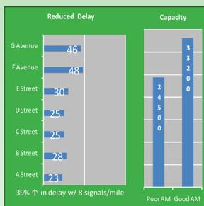
Increasing the distance between traffic signals improves the flow of traffic on major arterials, reduces congestion, and improves air quality for heavily traveled corridors. The appropriate spacing between signals for a particular corridor depends greatly upon the speed and flow of traffic, but anything greater than two signals per mile has a significant impact on congestion and safety.
