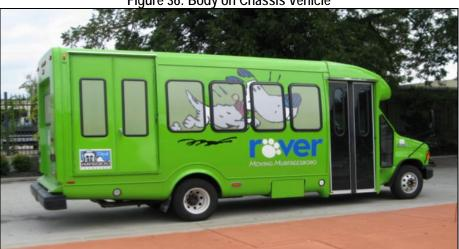
Figure 36: Body on Chassis Vehicle
